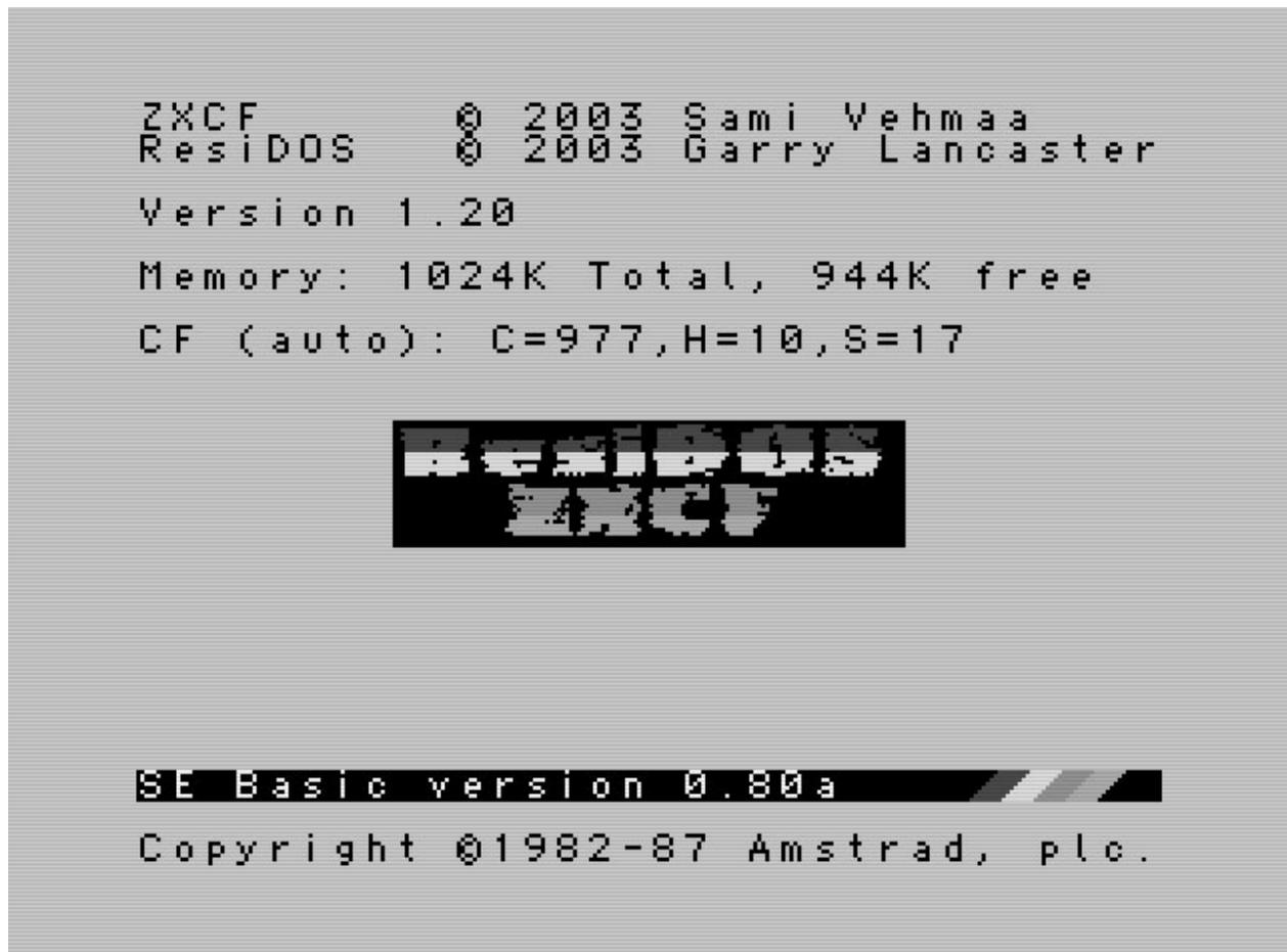
The RAM in your **ZXCF** or **ZXATASP** interface can be used to store alternative versions of BASIC, or Interface II ROM images. Once they have been added, you can start them up at any time using a simple command.
